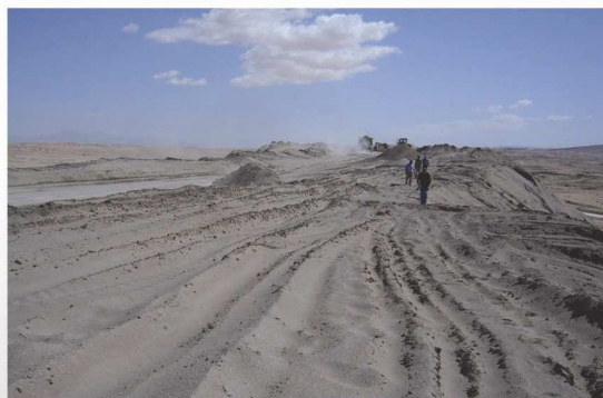
● Natural drying of phosphate in Metlaoui
